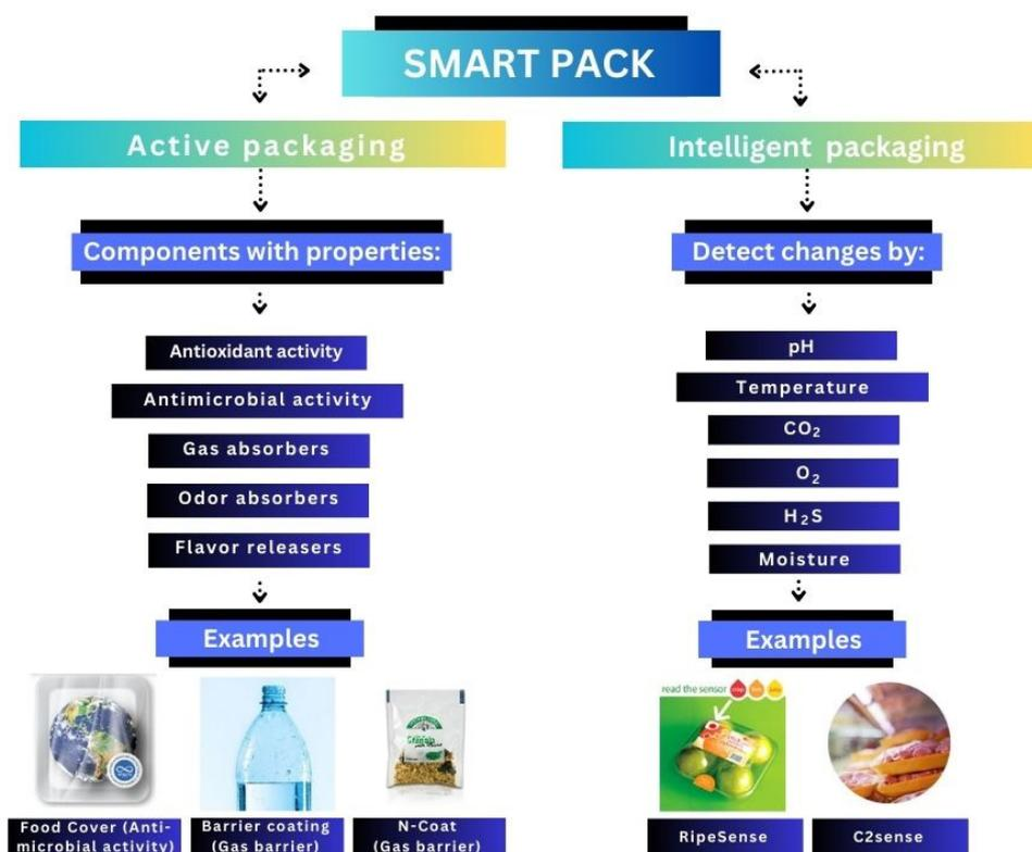
**Figure 1.** The two types of smart packaging, active and intelligent packaging, and their functions and examples.
