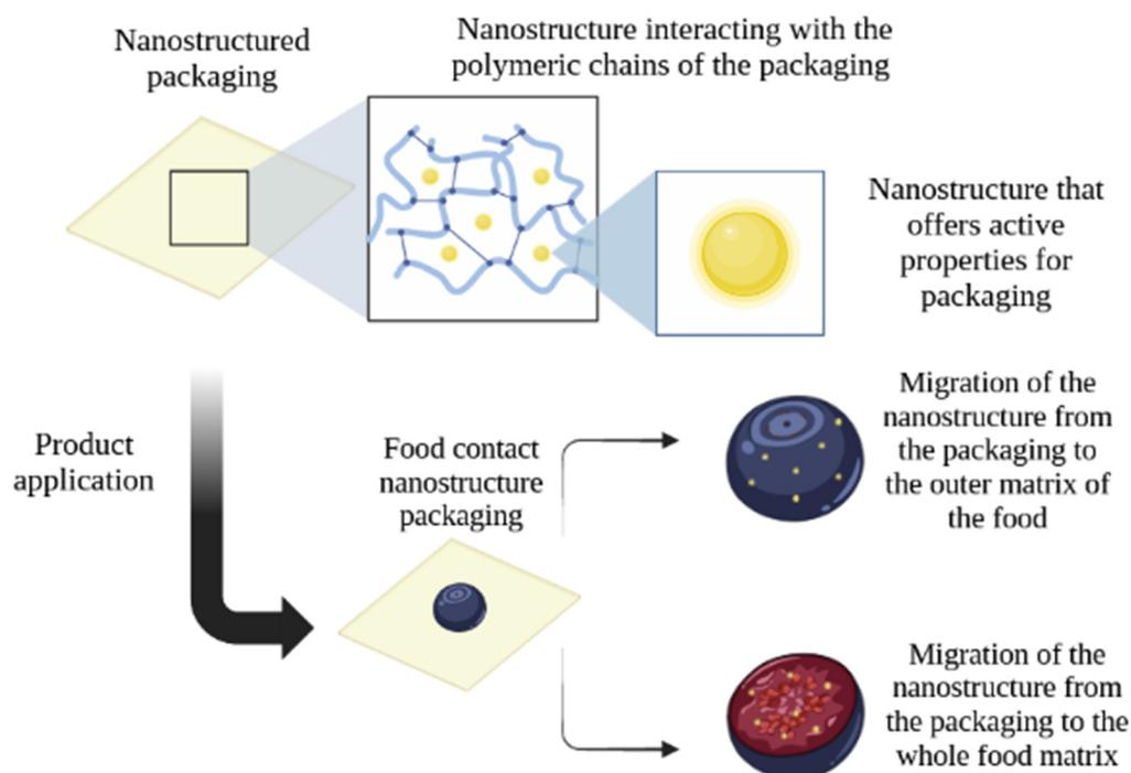
**Figure 3.** Migration of a nanostructure from a packaging surface to food. Created in [BioRender.com](https://www.biorender.com).
